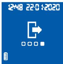
To move through the different menu options, press the right button. To execute the desired option, press the left button. You can exit the Bluetooth menu at anytime by inserting a microINR Chip or after 20 seconds of inactivity the Meter will skip the menu automatically.
