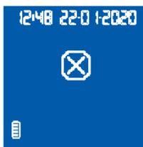
Once the pairing process starts, the microINR Link Meter is accessible for 60 seconds to pair with a compatible device. If the microINR Link Meter does not connect with another device, the “*Process Incorrect*” symbol will appear. The “*Unpaired Device*” symbol will appear on the lower right side of the screen.
