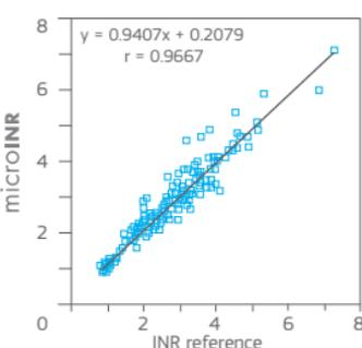
If the system has been handled correctly by a trained user, at least 90% of the times the microINR system's result will differ a maximum of ±30% from the laboratory test value.
